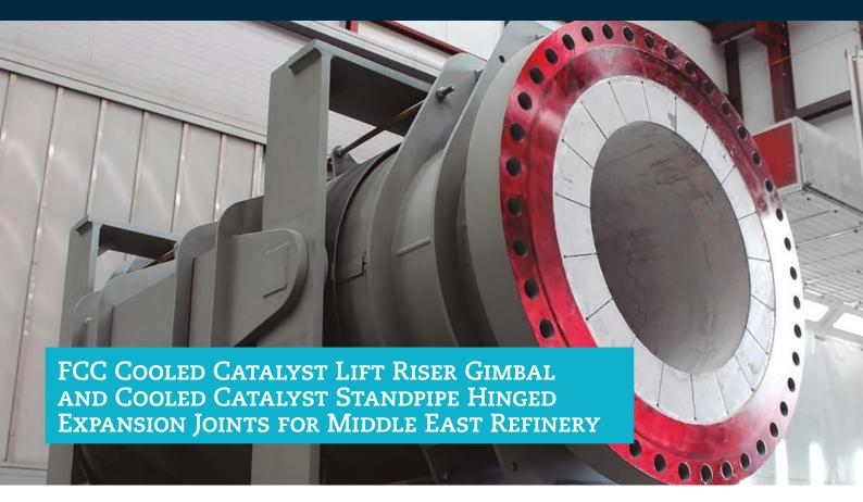
The scope of supply included complete detail design, fabrication, preparation and application of refractory linings and testing in accordance with UOP project & standard specifications.
