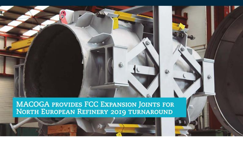
The MACOGA scope of supply included complete detail design, fabrication, preparation and application of refractory linings and testing in accordance with UOP standards and project specifications.
