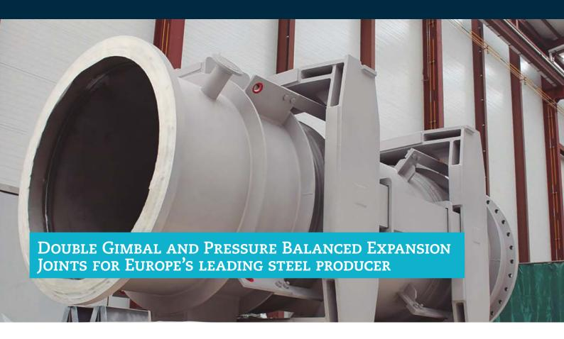
We have designed, manufactured, tested and shipped several high-tech Double Gimbal, Pressure Balanced, Universal Restrained and single Hinged Expansion Joints for Europe's leading steel producer.
